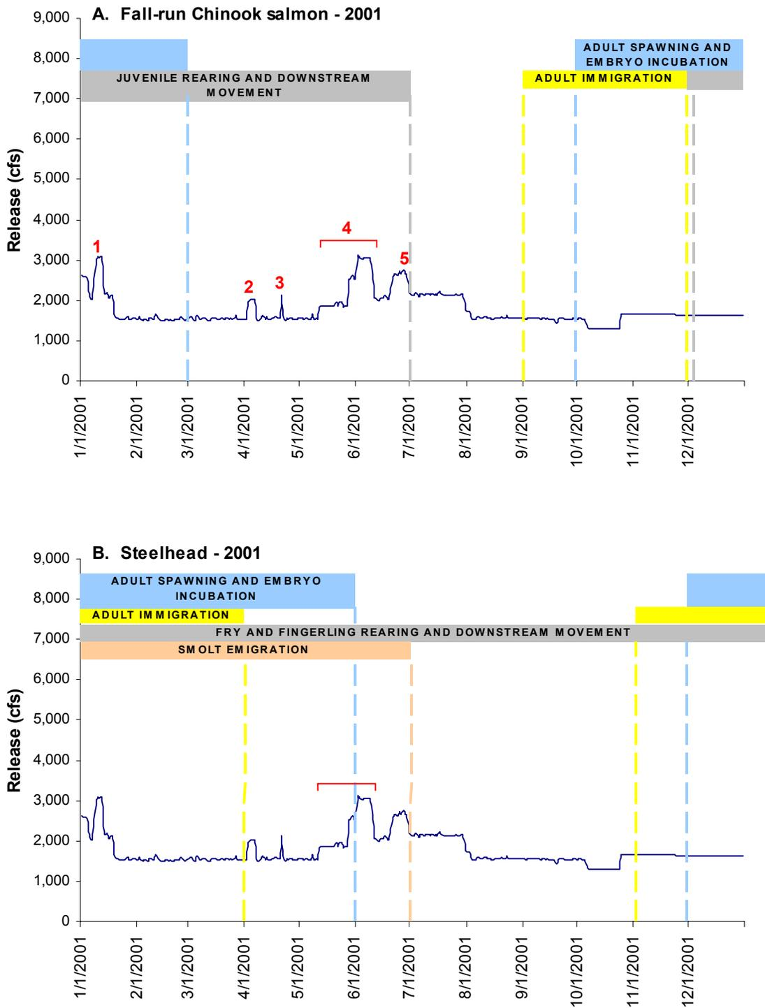
**Figure 1. Mean daily release rates from Nimbus Dam in 2001. The life stage timings for fall-run Chinook salmon (A) and steelhead (B) are displayed. Sequential red numbers indicate release events attributed to either Delta water quality objectives or Delta demands in Reclamation’s Nimbus Dam release logs.**
