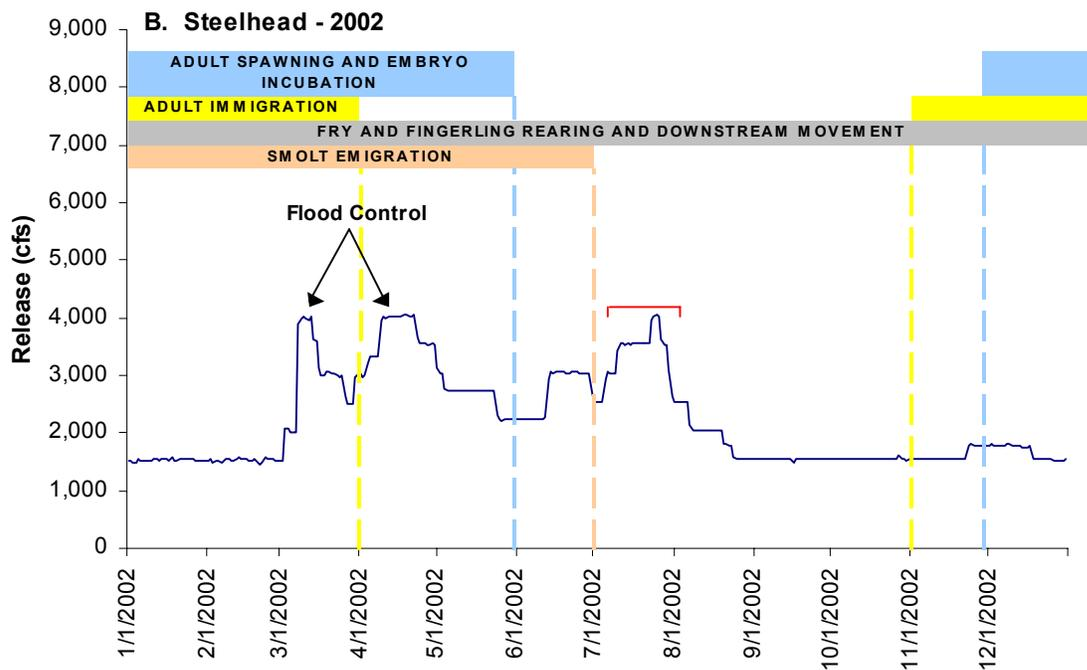
**Figure 2. Mean daily release rates from Nimbus Dam in 2002. The life stage timings for fall-run Chinook salmon (A) and steelhead (B) are displayed. Sequential red numbers indicate release events attributed to either Delta water quality objectives or Delta demands in Reclamation's Nimbus Dam release logs.**
