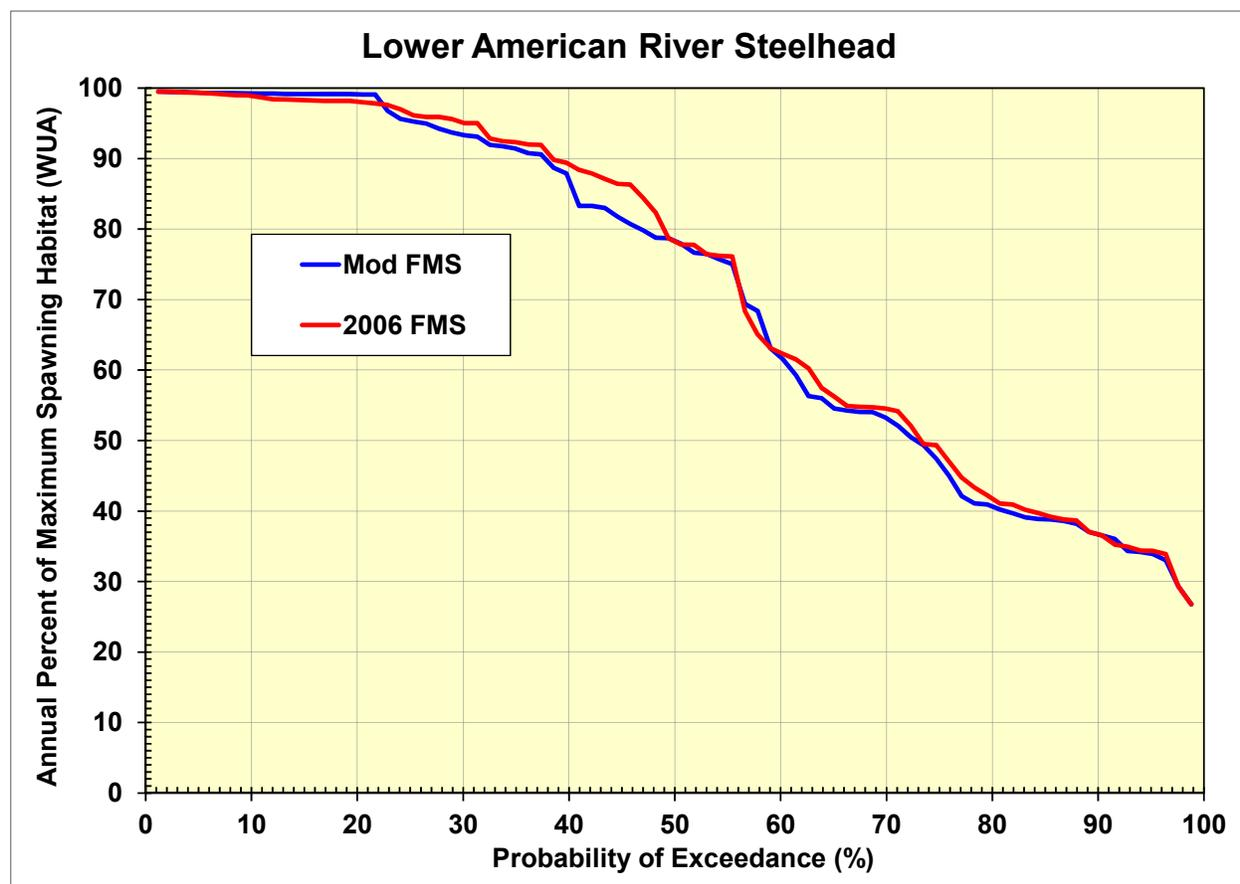
Figure 26. Comparison of steelhead spawning habitat duration over the 82-year hydrologic simulation period for the Modified FMS and 2006 FMS scenarios.
