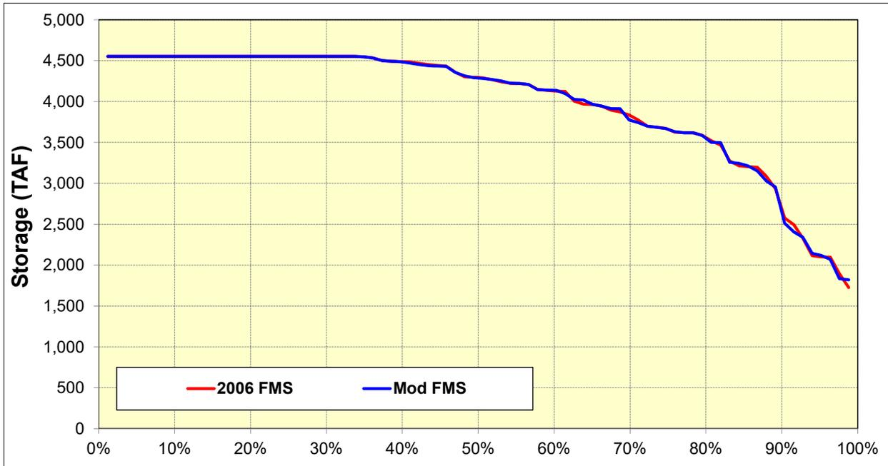
Figure F-1. Exceedance plot of May Shasta Reservoir storage for the Modified FMS and the 2006 FMS for the 82-year period of evaluation.
