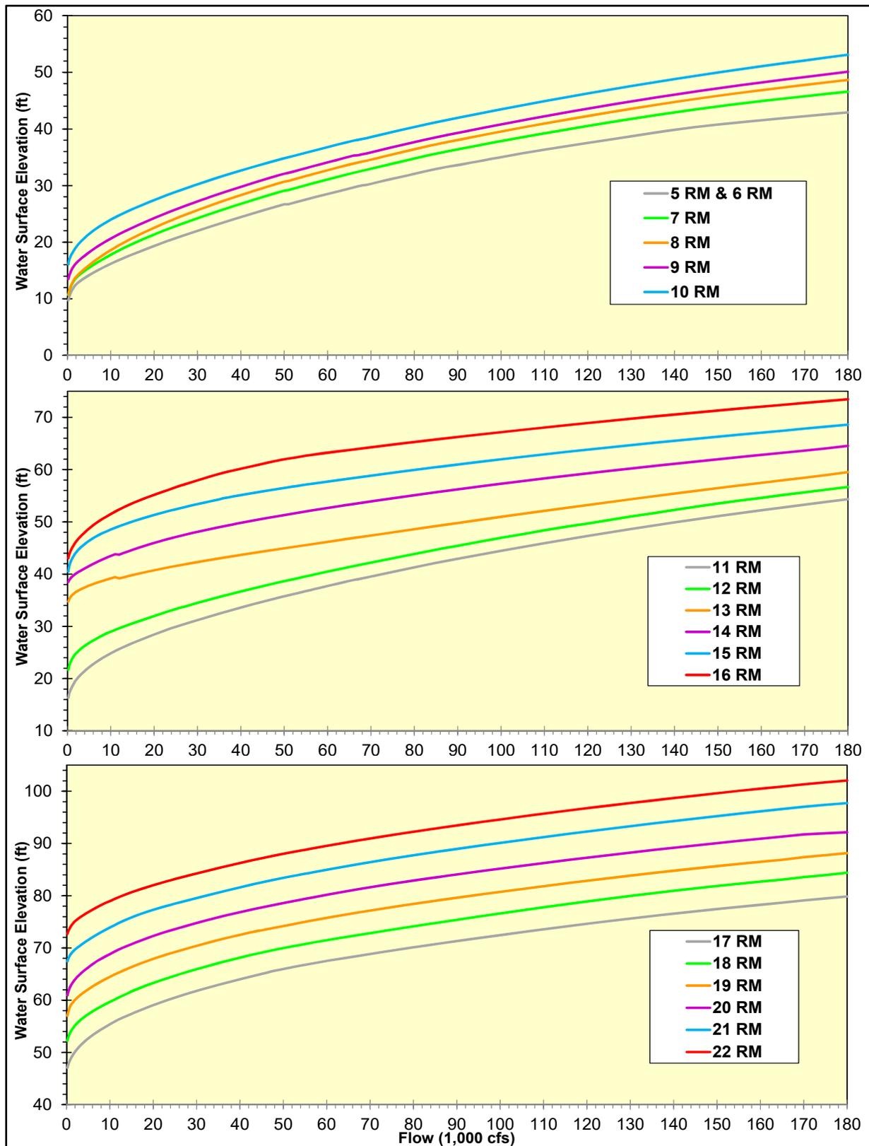
Figure C-9. Relationships between water surface elevation (ft) and flow (thousand cfs) developed by cbc for each of the 18 spawning reaches used in the redd-dewatering analyses for Chinook salmon and steelhead in the lower American River.
