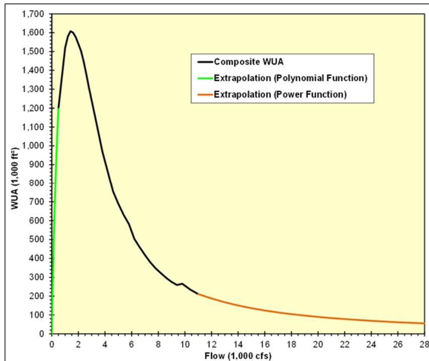
**Figure B-20. Final relationship between the composite WUA and flow for steelhead spawning in the lower American River.**
